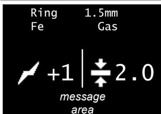
In Synergic Mode, the time and current for the different phases are selected automatically by the machine.
