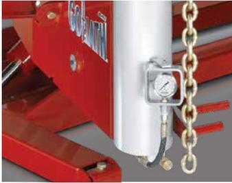
**Individually mounted pressure gauges and shut-off valves keep clutter to a minimum**
