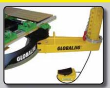
Pulling towers remain attached to the bench and effortlessly glide 360 degrees around the bench. The "Vector" design of the towers means chain angles are always correct for every pull.
