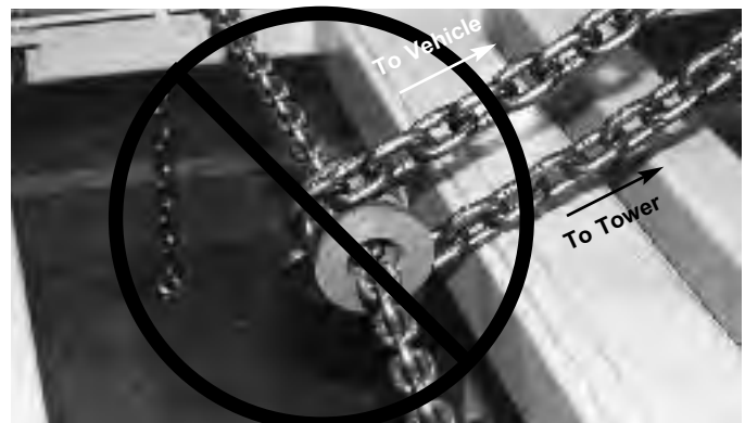
Do not use Down Pull Attachment in this manner. See CAUTION No. 2 above. Also refer to Figure 6 below.
