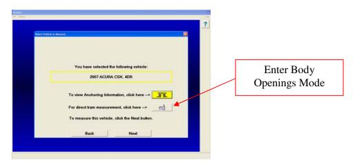
• If you are currently measuring with a scanner, click the Red X to stop the scanner mode. Click the **TRAM** icon in the bottom right corner of the screen.
