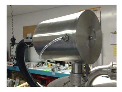
c. Remove the used coalescing filter element (CFE) and install a new coalescing filter element (CFE).
