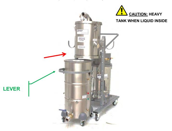
i. Make sure the black connection hose between the vacuum cleaner and the wet mix immersion separator is connected.
