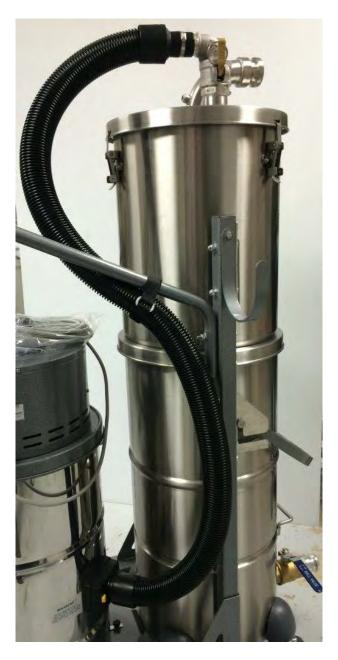
j. Connect the airline hose of one or two static conductive suction/air hose to the air outlets placed on the vacuum cleaner
