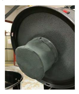
c. Unscrew and remove the acorn nut and the rubber washer securing the HEPA filter.
