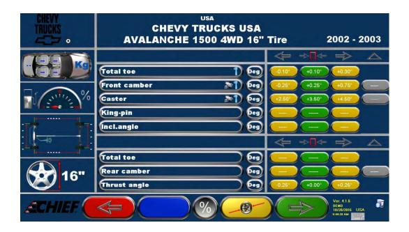
Remote operation....Computer console can be stationed anywhere in the workshop...System is operated remotely by phone or tablet. No dedicated service lane is required! The FastCheck system goes to the vehicle instead of the vehicle being required to come to the test system. Fastchecks can be done on one or both axles.
