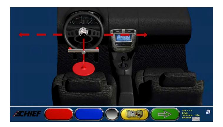
After completion of turning routine operator is prompted to apply steering wheel lock.
