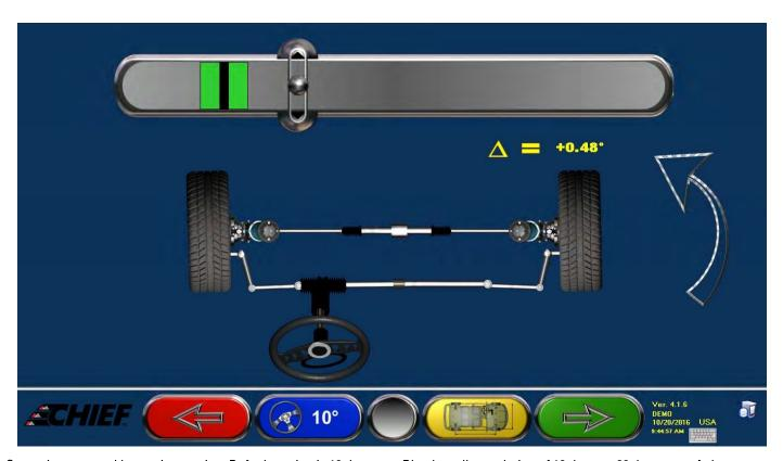
Caster is measured by turning routine. Default setting is 10 degrees. Blue key allows choice of 10 degree, 20 degree, or Ackerman angle. Turn left until pointer is on the target.
