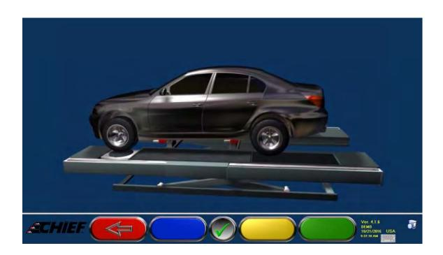
Make adjustments with vehicle raised. When adjustment procedure is done select blue key to lower the vehicle. When vehicle is back down on the platforms confirm using F5 key or the center black key on the measuring head or on the phone.
