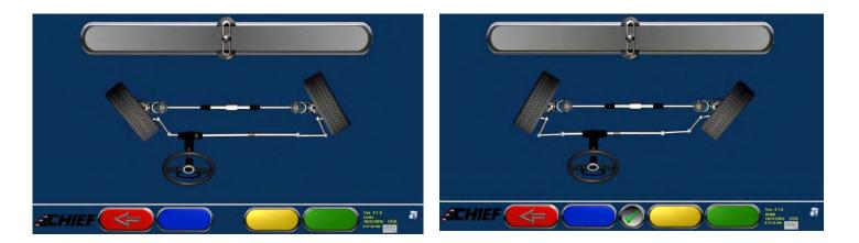
Steer left then right to equalize pressure in the steering system. Position steering wheel in desired straight position then select F5 or black center button on sensor head or on smartphone to confirm.
