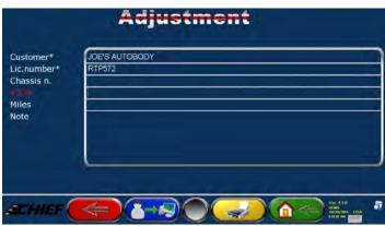
Select green to advance to the summary screen. Then select yellow (printer icon) to move to the customer information page. Note: Customer information can also be entered at the beginning of the alignment procedure. Note: Fields indicated by an asterisk \* must be completed.
