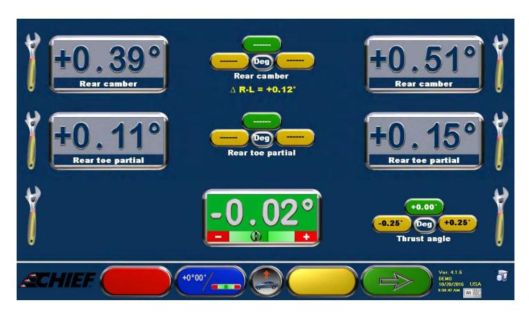
Rear Axle Adjustment Screen is live. Wrenches in the side margin indicate this is a live adjustment screen. Blue key allows you to change screen view.
