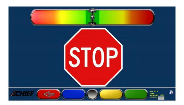
Alignment specifications are displayed for operator's review. Select Green and move forward. Steer to straight ahead.
