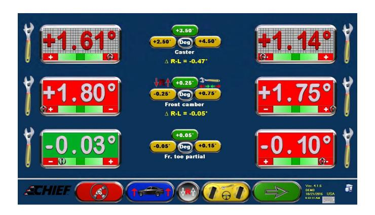
Application for setting front toe when wheels need to be steered away from center due to a lack of space. Also used when operator prefers not to use the steering wheel lock. Select this feature with the yellow key.
