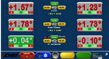
Select either right or left wheel to begin by choosing the blue or yellow key. The snowflake icon on the key indicates that the side not chosen will be frozen so that its toe values remain unchanged. The side chosen will become "live" and the grid will be removed from that adjustment box.
