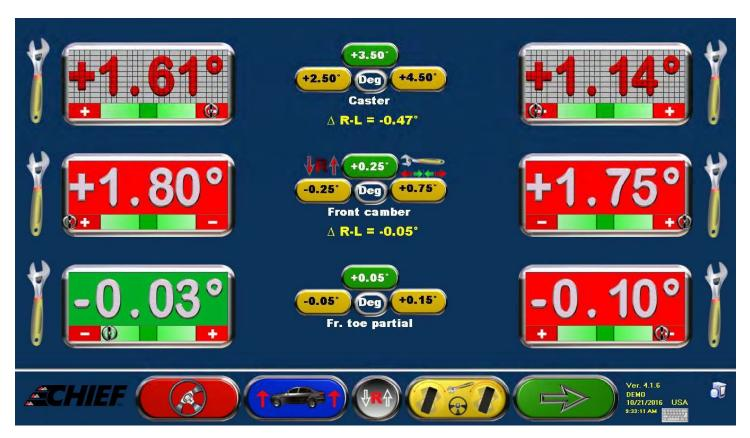
Front adjustment screen with live caster, camber, and individual toe. To access total toe bar graph select Shift/F5 from the keyboard.
