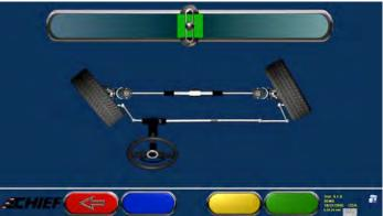
Select red key for final steering procedure. Steer to position wheel in the desired straight position. Select F5 on the keyboard or the black key on the sensor head or smartphone to confirm.
