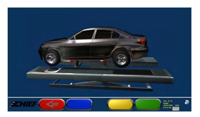
Raised mode can be used for front or rear axle. Select the blue key to enter raised mode. Once vehicle is raised and supported by jacking beam confirm with F5 key or by pressing center black key on sensor head or on the Smartphone.
