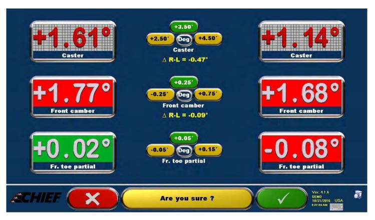
To progress from the measurement stage to the adjustment phase of the program simply select green to confirm.
