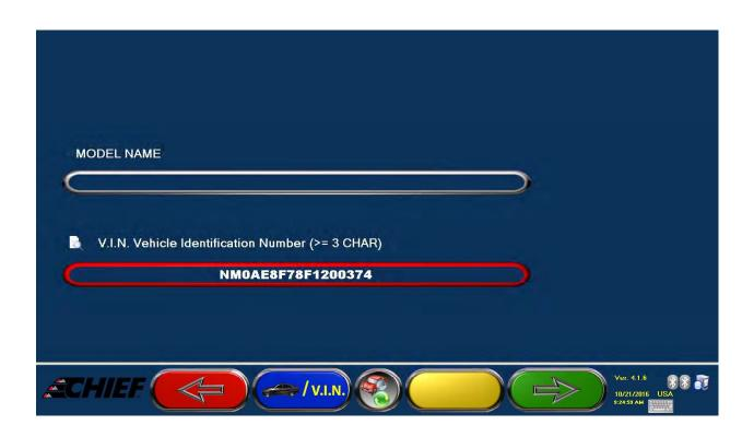
Select vehicle using the VIN scanner or typing the VIN into the designated field. Vehicle can also be selected by make, model, and year.
