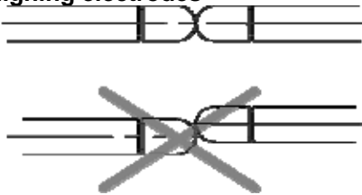
Fig.36: "Electrode must be in true alignment"
