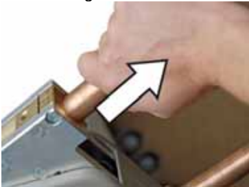
Fig.31: Removing the electrode arm.
