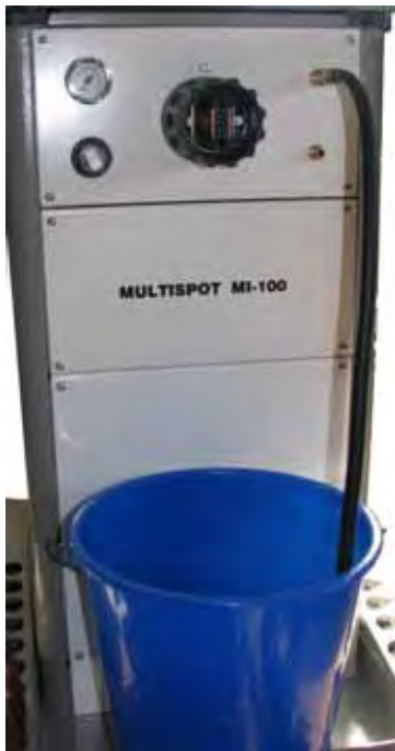
Fig.57: Draining cooling water.
