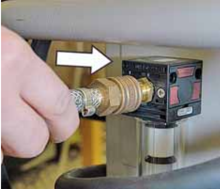
Fig.24: Connecting compressed-air supply
