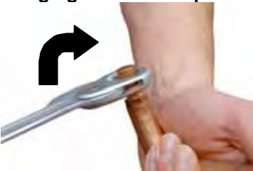
Fig.32: Exchanging electrode caps
